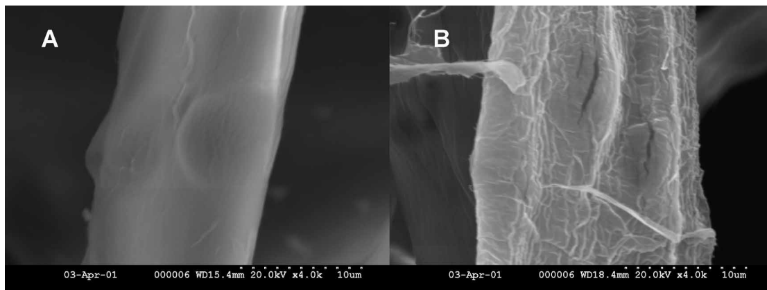
FIG. 3. Scanning electron micrographs (SEM) at 4,000 \times magnification of pulp fibers generated from (A) control wood chips and (B) fungal pretreated wood chips.
