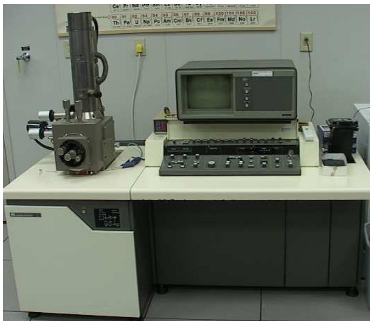
Figure 5.2 Photograph of International Scientific Instruments WB-6 scanning electron microscope during this research.
