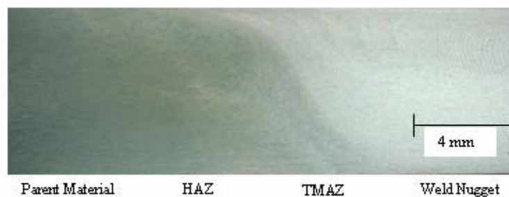
Figure 3 A Cross section of the welded specimen
