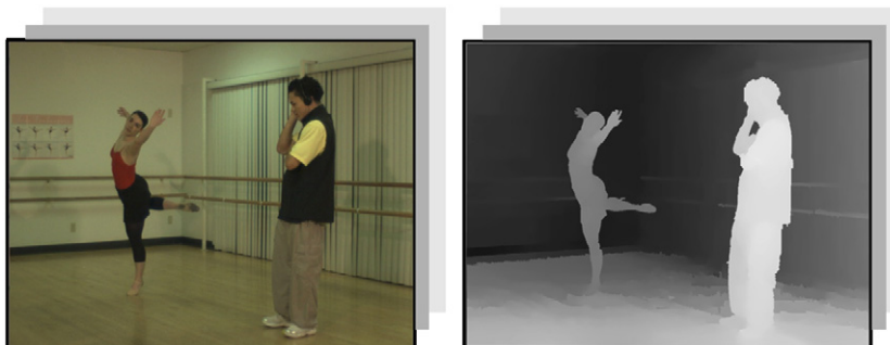
Fig. 1. Example for the MVD format with texture images (left) and corresponding depth-images (right). A typical depth-image frequently contains regions of linear depth changes bounded by sharp discontinuities.
