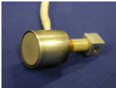
Figure 3 – Photograph of the JPL nude Faraday probe.
