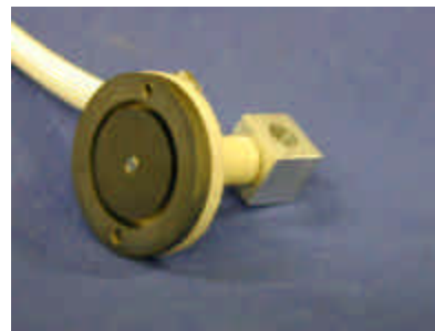
Figure 5 – Photograph of the GRC nude Faraday probe.
