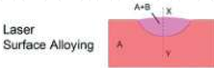
Figure 3. Schematic diagram displaying laser surface alloying [15].
