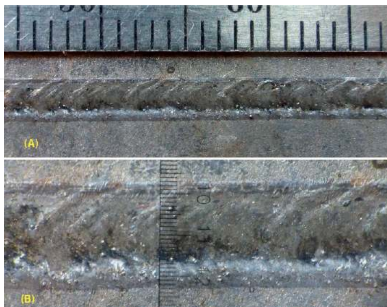
Figure 10. Top view of a laser-generated coating on weld bead [26].
