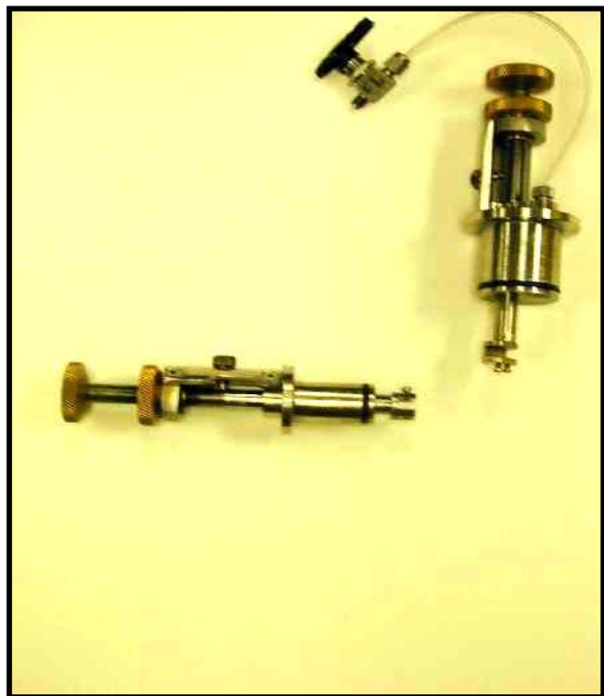
Figure 7(b): Close-up View of the Upper and Lower Crystal Holders
