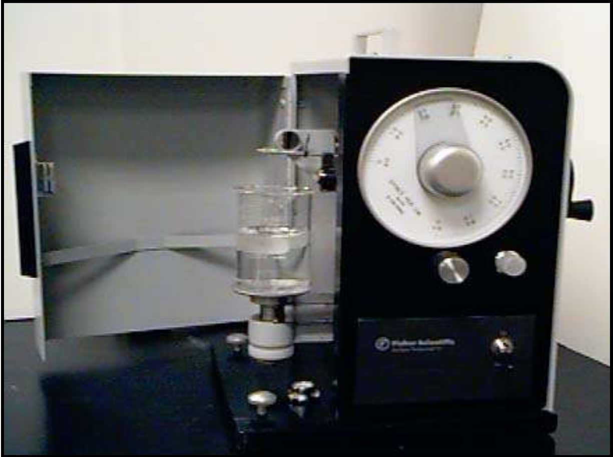
Figure 12: du Nuoy Ring Tensiometer for High Interfacial Tension Measurements
