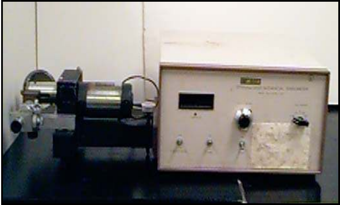
Figure 14: Spinning Drop Interfacial Tensiometer for Low Interfacial Tension Measurements
