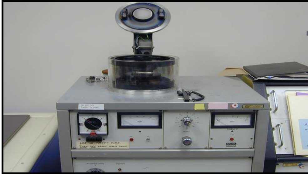
Figure 15: S-150 Sputter Coater for coating the rock surfaces with gold and palladium
