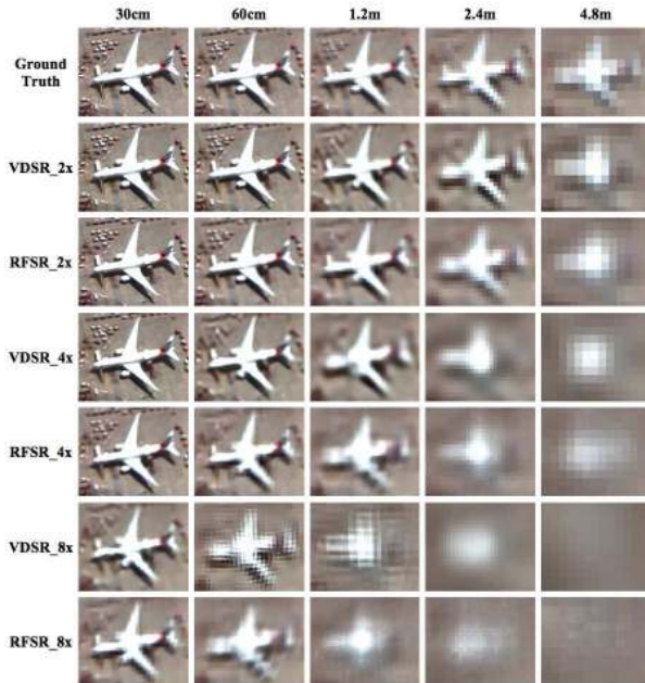
Figure 3: The effects of super-resolution on a plane and neighboring objects. As resolution degrades super-resolution becomes a less tractable solution.
