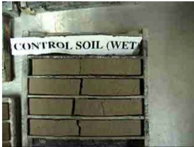
Figure C.1 Linear Shrinkage Mold of Control Soil at Optimum Moisture Content
