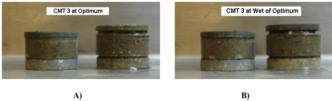
Figure 4.8 CMT 3 Samples – Before and After Swell Tests A) Optimum Moisture Content and B) Wet of Optimum Moisture Content
