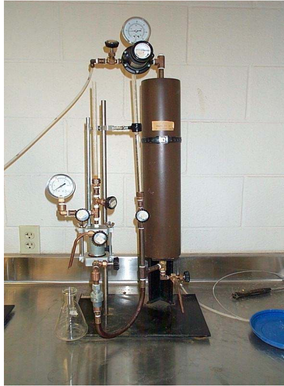
Figure 3.6 Permeability Test Setup
