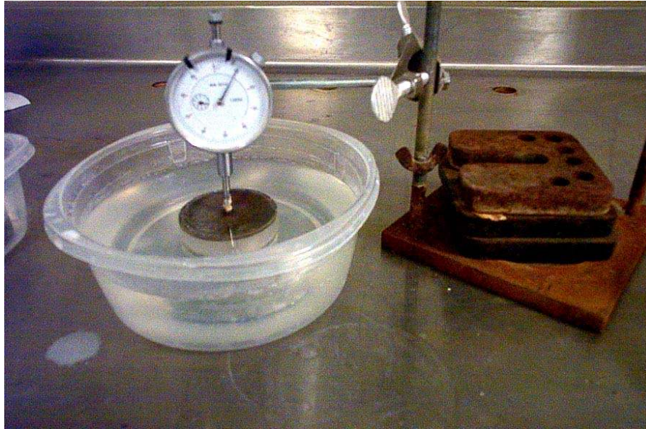
Figure 3.2 Laboratory Setup of One-Dimensional Free Swell Test
