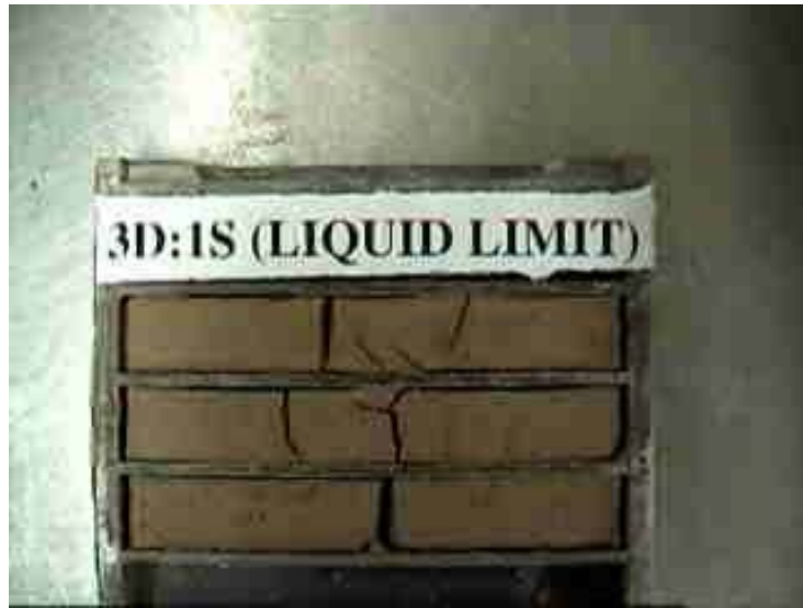
Figure C.5 Linear Shrinkage Mold of CMT 1 (DM_75) at Liquid Limit
