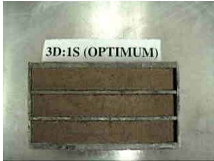
Figure C.3 Linear Shrinkage of CMT 1 (DM_75) at Optimum Moisture Content
