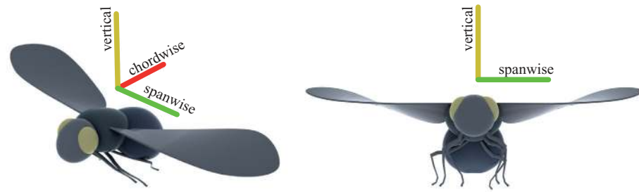
Figure 1. Wing twist at mid-downstroke in an insect. Wing twist is the torsion of a wing along the spanwise axis, leading to a variation of the geometric angle of attack over wing span. Left: perspective view. Right: frontal view.
