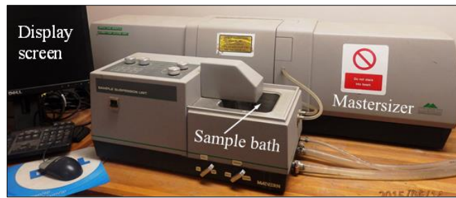
Figure 3.19: Soil gradation analyser: Malvern 3B Master-sizer (Courtesy: UOW)
