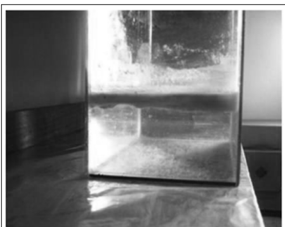
Figure 1 - Phase separation after treatment by electrocoagulation. The example shown was performed under the conditions of the test at optimized condition.
