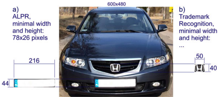
Fig. 2 Proportions of car number plate and logo objects within the 600 \times 480 FOV and their minimal required resolutions—with respect to (a) [9] and (b) [15]
