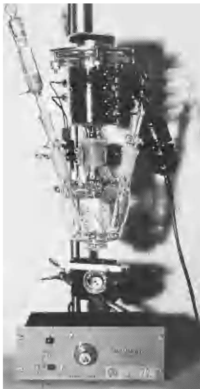
Figure 3. Rotating ring-disk electrode assembly for use in aprotic solvents and closed systems. The entire motor-tachometer assembly is enclosed in the glass envelope. The motor power supply and controller is at the bottom of the picture
