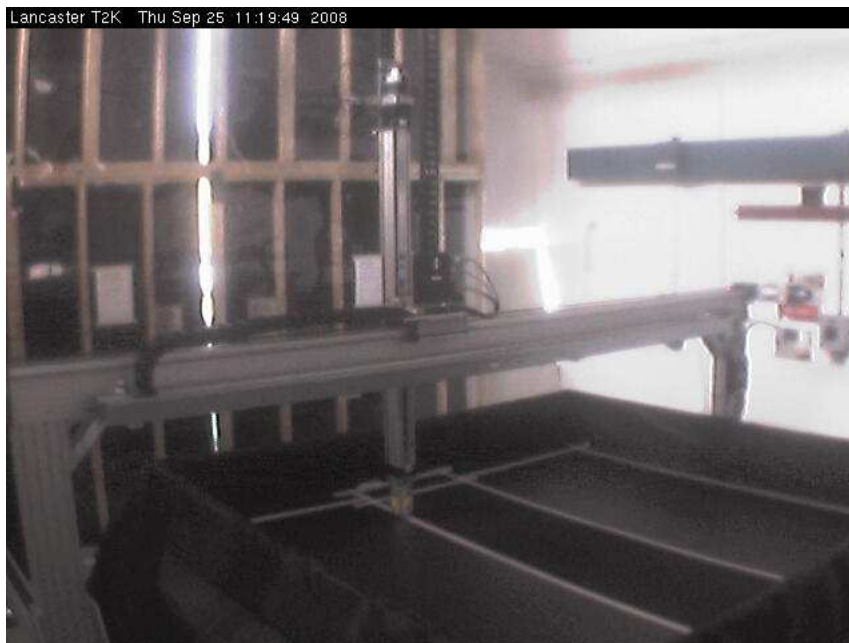
Figure 14. The 2D scanner moving along the scintillator bars in the Ds-ECal. The ^{137}\text{Cs} source sits at the bottom of the vertical arm of the scanner, just above the layer being scanned. The blackout material covering the layer is seen, along with the tape holding it in place for the duration of the scan.
