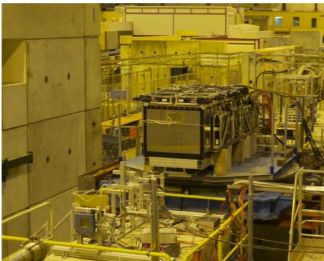
Fig. 1. The new SuperDREAM fiber calorimeter, installed in the H8C beam area. The system of trigger counters and beam defining elements is visible in the left bottom part of the figure.
