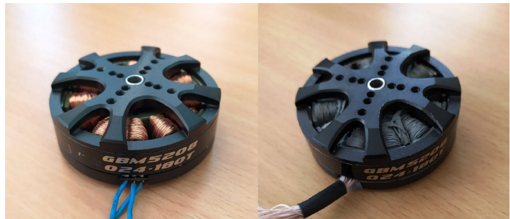
Figure 4. Original and modified motors GBM5208—original (left) and modified (right).
