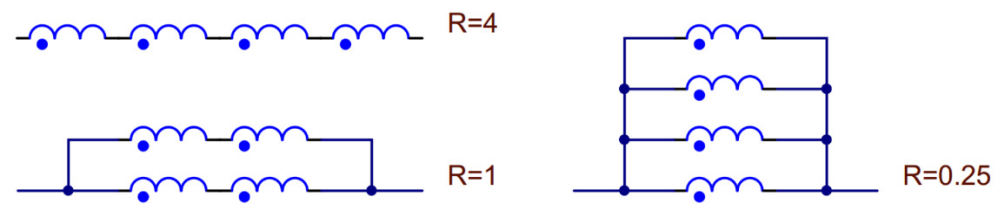
Figure 3. Possible connection schemes for four poles.
