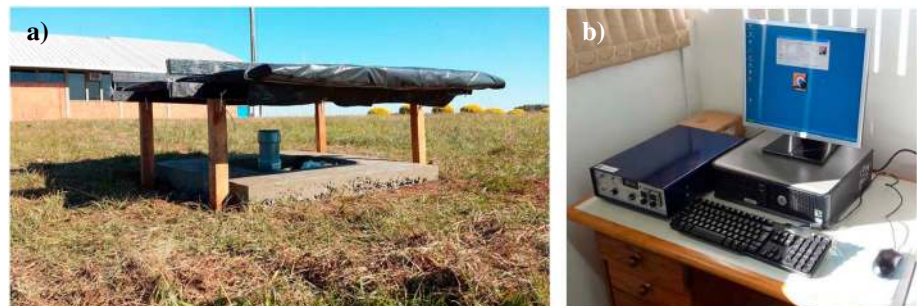
Figure 6. Picture of (a) the magnetic sensor buried 1 m deep under a wood shelter and (b) the system controller with the personal computer for local data storage, and Internet FTP server at the SMS station.
