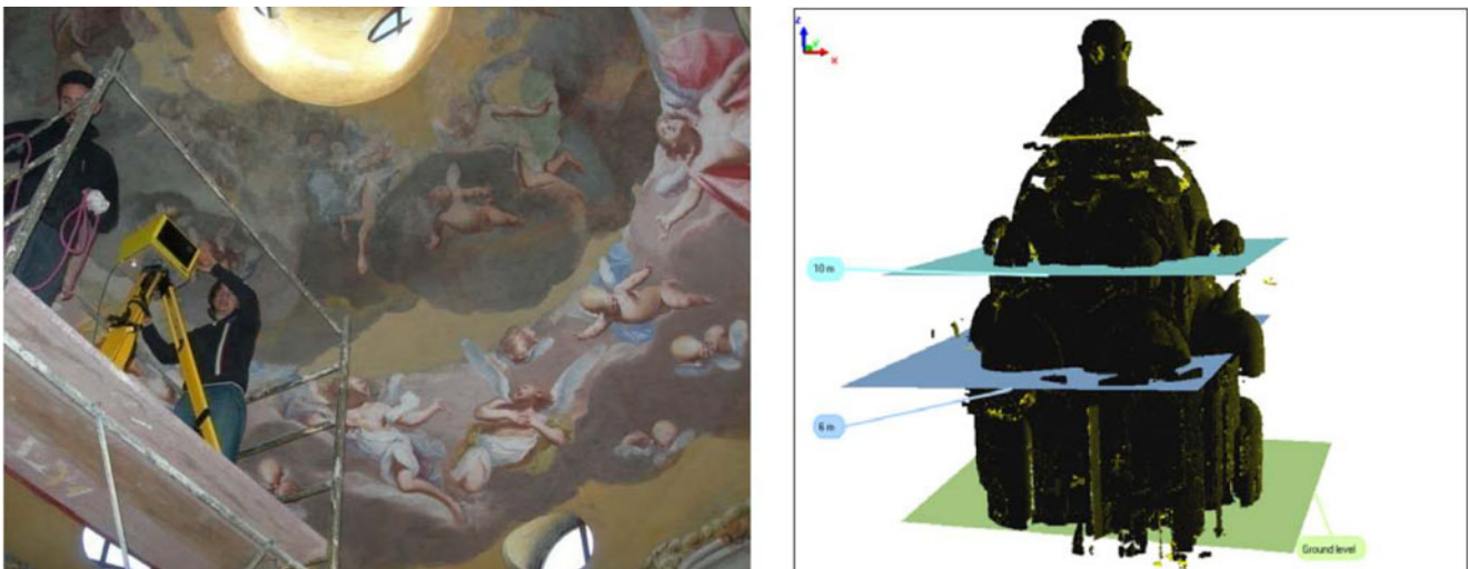
Fig. 3 Interior survey ( left ) and scaffolding levels ( right )
