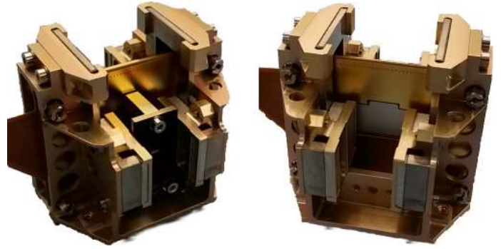
Fig. 7. Assembly of the STEP Magnet Channel detector with ( left ) and without ( right ) front pinhole.
