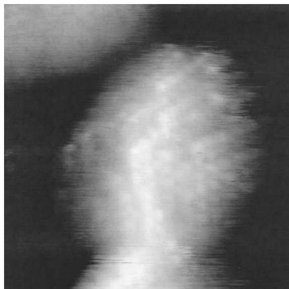
Fig. 7. An 11 \times 11 -nm STM image of a palladium particle, with atomic resolution [475]. Reproduced with permission from [475].
