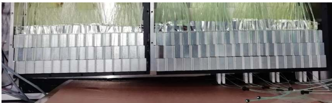
Figure 8. Four doublets of the photon veto installed below Module 3 (bottom rightmost part of the figure).
