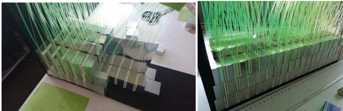
Figure 5. Mounting of one of the Modules before the bundling of the fibers and the installation of the SiPMs.
