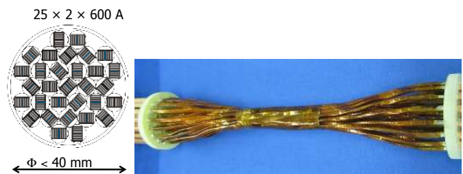
Fig. 5. Left: cable with 25 channels of twisted pairs for 600 A. Right: short test piece of YBCO tape twisted pair cable.
