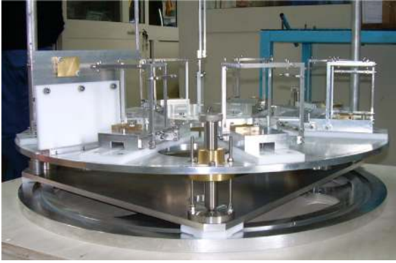
Fig. 5. The supports of the telescopes are mounted on Derlin platforms (in white color) placed on a rotating aluminum table. This table separates horizontally the reaction chamber in two volumes: the upper volume and the lower one (see also Fig. 7 that illustrates a schematic view of the reaction chamber).
