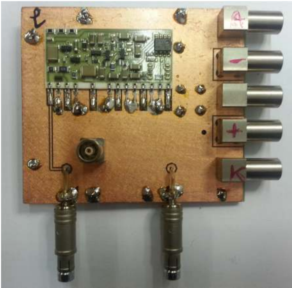
Fig. 8. PCB of the IC charge-sensitive preamplifier that is mounted on the IC vessel.
