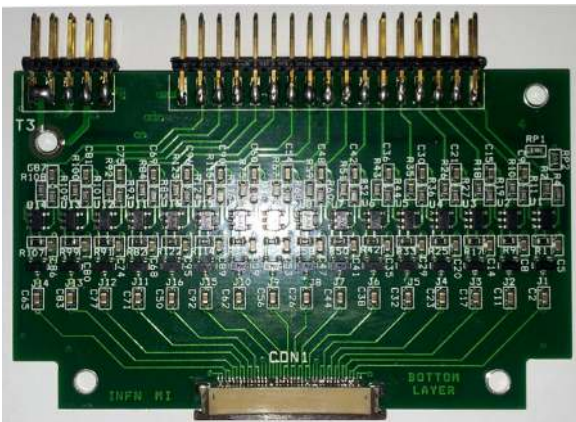
Fig. 9. PCB housing 16 charge-sensitive preamplifiers for the electronic readout of signals originating from one side of the 40/60 \mu m-thick DSSSD detector (16 channels/side). The ERNI 36-pin connector, where the input Kapton cable is inserted into the PCB, is located on the PCB bottom part. The board power supply connector (left) and the output signal connector (center) are placed on the PCB upper part.
