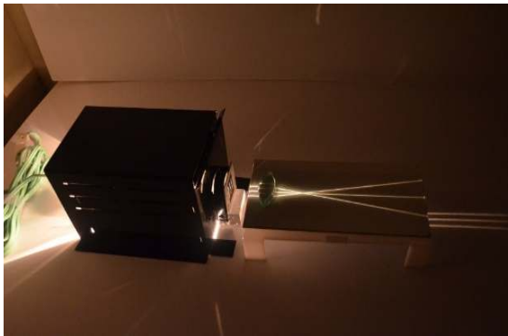
Figure 18. Parallel beams crossings or converging in the focus of the biconvex lens
