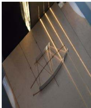
Figure 33. Beams directed to focus of the parabola
