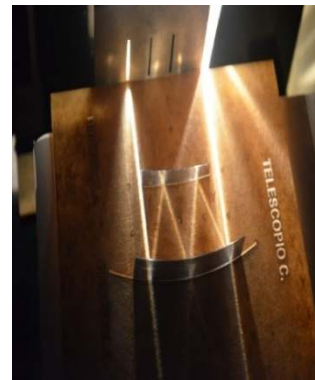
Figure 30. The Cassagrain telescope physical concept representation
