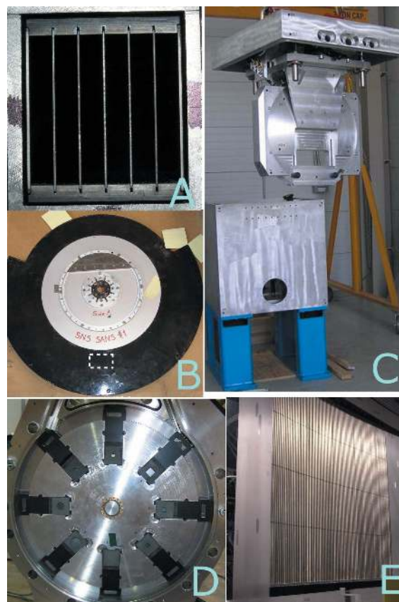
Figure 2 Selected EQ-SANS components. A: Neutron beam bender in the primary beam shutter. B: Bandwidth chopper disc. The dark area is coated with neutron absorber ( ^{10}\text{B} ), and the dashed line indicates the cut-off option for a future high-speed upgrade. C: Bandwidth chopper housing with a dummy chopper attached to the lid. The chopper can be translated up and down by 10 cm. D: Slit selections on the collimation slit wheel. E: The low-angle detector array. See text for full details.
