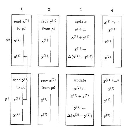
Figure 3.10: Two-Track Implementation of the Distributed GS Butterfly
