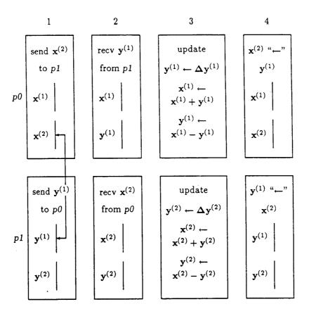
Figure 3.11: Two-Track Implementation of the Distributed CT Butterfly
