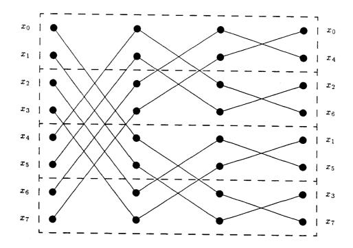
Figure 3.3: n = 8, P = 4, signal flow graph (GS1, CT1)
