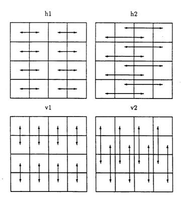
Figure 4.7: Block Method 2D-FFT Communications for a 16-node hypercube
