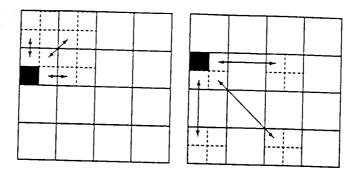
Figure 4.8: Vector-Radix Exchanges for Processor p0100
