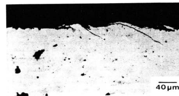
Fig. 9 Section through a fretted region of a peened alloy
