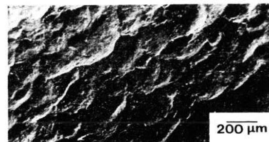
Fig. 1 Scanning electron micrograph of the peened surface
