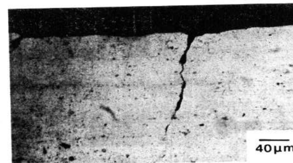
Fig. 8 Section through a fretted region of a non-peened alloy
