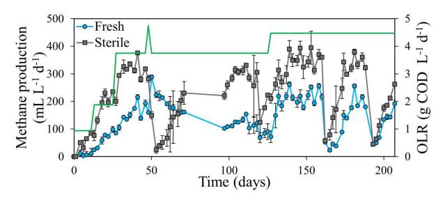
Figure 1 Methane production in function of time in the digesters fed fresh and sterile waste
