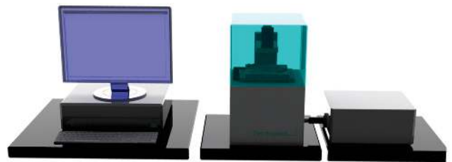
Fig. 3 Artistic view of the prototype Femtoprinter. The system consists of a control unit, a laser scanning system (central part) and the laser source (right).
