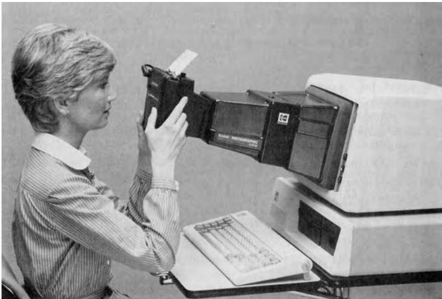
Fig. 4. Kodak Instagraphic CRT print imager illustrated in John Lewell, A-Z Guide to Computer Graphics (1985)
