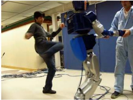
Fig. 7. Impact test of HRP-2P
