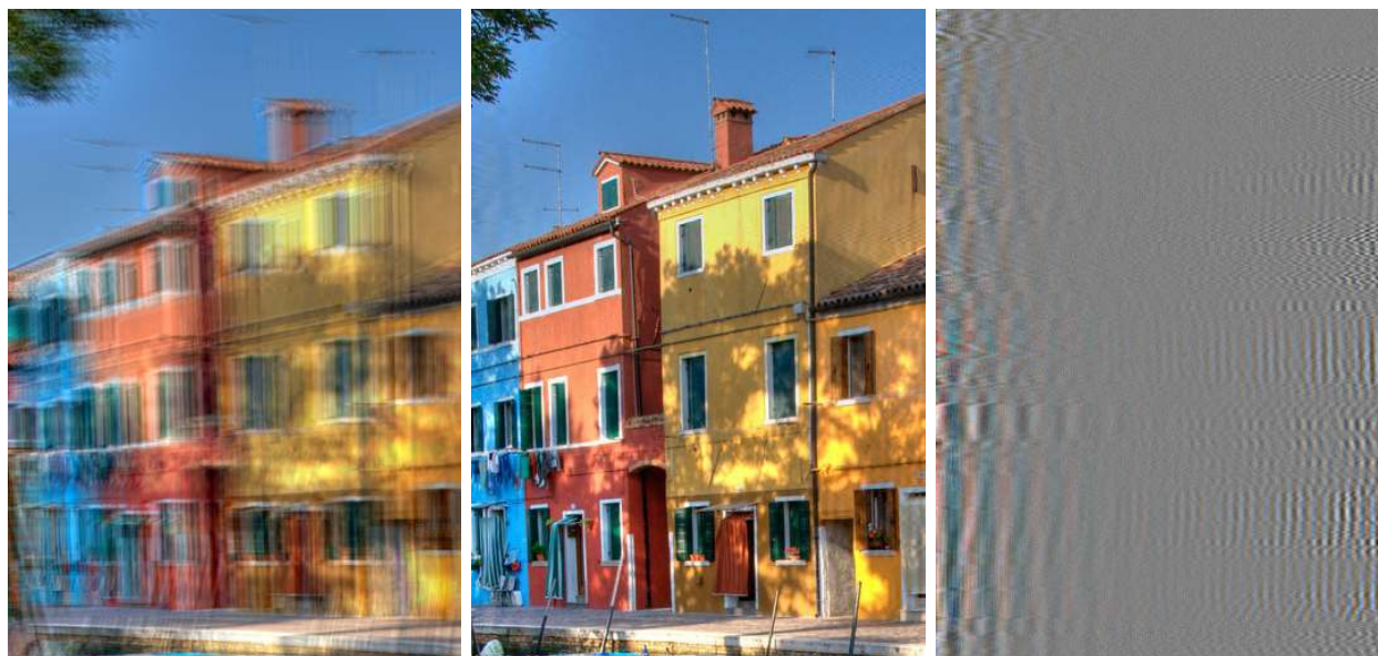
Figure 12: Random code. Left: observed image. The blur interval length is equal to 52 pixels here. Middle: reconstructed image (RMSE = 2.01). Right: residual noise (difference between ground truth and reconstructed, dynamic normalized on [0, 255] by an affine contrast change).
