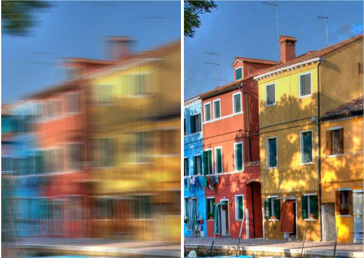
Figure 1: Left: simulated observed (blurry and noisy) image, notice the stroboscopic effect of the flutter shutter apparatus. The blur interval length is 52 pixels. Right: reconstructed image (RMSE = 2.55). Such reconstruction is not possible without a flutter shutter camera.
