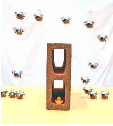
Fig. 2: A sequence of photographs demonstrating the multi-modal trajectory tracking capability of the flying monkey.
