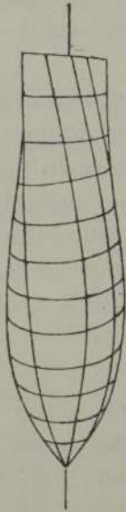
FIG. 7. — Body with circular cross-sections in lower half, finishing in a point \epsilon , and elliptical cross-sections in upper half with knife-edge on top.
