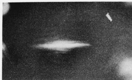
FIGURE 12. Optical micrograph showing an edge-on view of a multilayered crystal formed in a T_c = 140^\circ\text{C} preparation which has been filtered and washed at 140^\circ\text{C} prior to cooling to room temperature.
