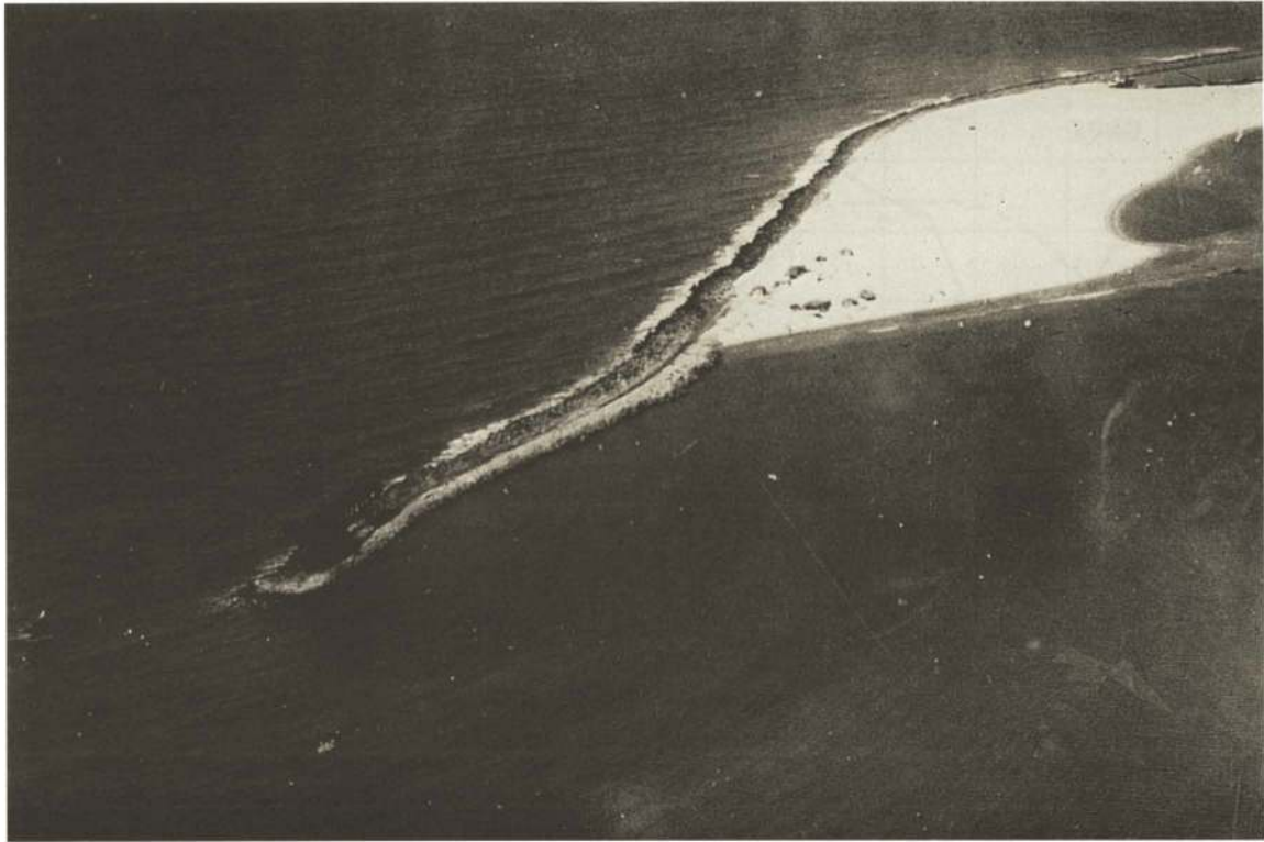
Figure 6. Sediment deposition in the leeward side of Port of Mucuripe around 1950.
