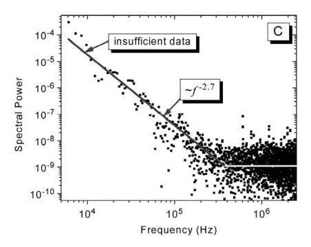
Fig. 3 As figure 2 but for a carbon arc pulse; the white noise extend to lower frequencies in this case.
