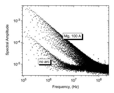
Fig. 4 Average of 16 FFT curves of the burning voltage measured for pulsed magnesium arcs (100 A, 50,000 points with 500 ps per data point in time domain). One can clearly see the power-law decay which is close to 1/f in this amplitude presentation, corresponding to  $\sim 1/f^2$  for the spectral power. To indicate the reason for white noise at the high frequency end of measurements, the same FFT and average procedure was applied to the zero line (no arc).
