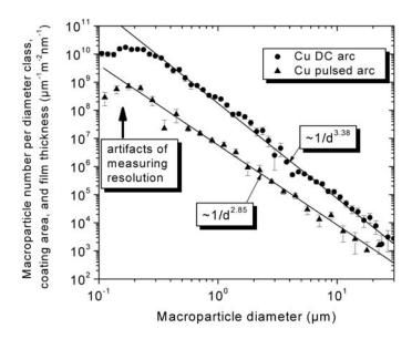
Fig. 5 Macroparticle size distribution for DC and pulsed copper arcs. The distributions show power laws indicating that a fractal dimension may be defined characterizing the dependence of the size distribution from experimental conditions.
