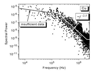
Fig. 2 Fast Fourier transform (power spectrum) of ion current for a copper vacuum arc (single pulse). One can see the approximate power law in the physically relevant interval.
