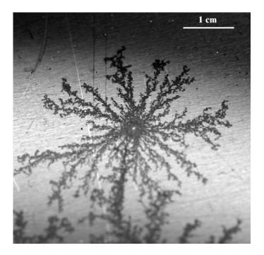
Fig. 1 Multi-spot arc traces on oxidized stainless steel.
