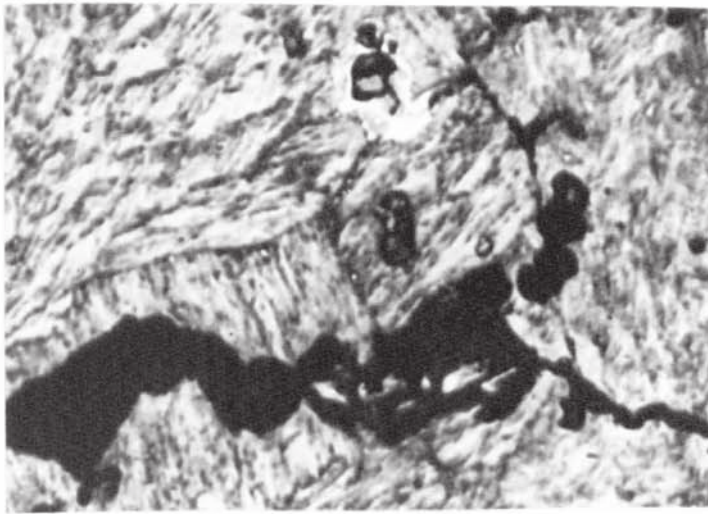
(b) Titanium sulphide adjacent to fracture path
