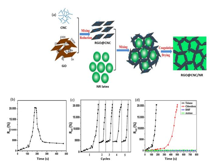
**Figure 14.** (a) Schematic illustration of RGO/CNC/NR with a 3D conductive network. (b) Responsivity—time relationship for RGO 2.08 vol% RGO/CNC/NR (b) when exposed to toluene the first time, (c) during five immersion-drying cycles and (d) when exposed to various interfering compounds. Reproduced from Ref. [118].
