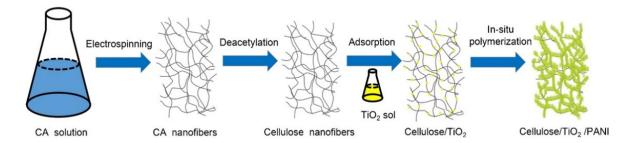
Figure 10. Production steps for CNF/TiO<sub>2</sub>/PANI composite. Reproduced from Ref. [116].
