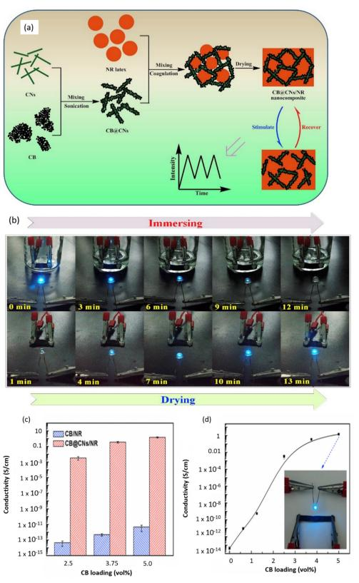
**Figure 13.** (a) Schematic presentation of 3D hierarchical conductive CB/CNC/NR fabrication. (b) Images of illumination change during CB/CNC/NR composite (5 vol% CB) immersion into toluene and drying by hot-air. Electrical conductivity responses of CB/CNC/NR and CB/NR with different volume fractions of CB (c), electrical conductivity of CB/CNC/NR as a function of CB content (vol%), (d) image of CB/CNC/NR lighting up an LED device by 9 V voltage (inset image). Reproduced from Ref. [117].
