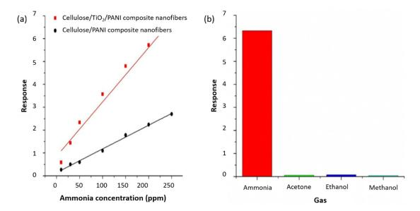
**Figure 12.** (a) Response of CNF/PANI and CNF/TiO<sub>2</sub>/PANI to various concentrations of ammonia (10–250 ppm), (b) Selectivity of CNF/TiO<sub>2</sub>/PANI in different solvent gases. Reproduced from Ref. [116].
