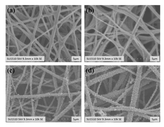
**Figure 11.** SEM images of CNF (**a**), CNF/TiO<sub>2</sub> (**b**), CNF/PANI (**c**) and CNF/TiO<sub>2</sub>/PANI composite (**d**). Reproduced from Ref. [117].
