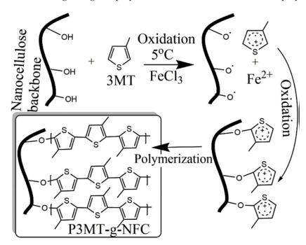
**Figure 9.** Grafting and polymerization mechanism between polythiophene and CNF. Reproduced from Ref. [108].
