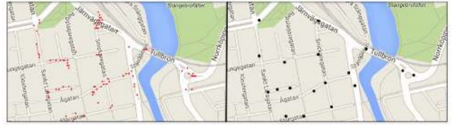
Fig. 3: There are different sensors in a modern vehicle that can detect potholes. Reports from a fleet of vehicles from NIRA Dynamics are sent to a cloud database (left fig), [23]. Since their notion of position differs for natural reasons (based on GNSS), clustering is needed in the cloud (right fig).
