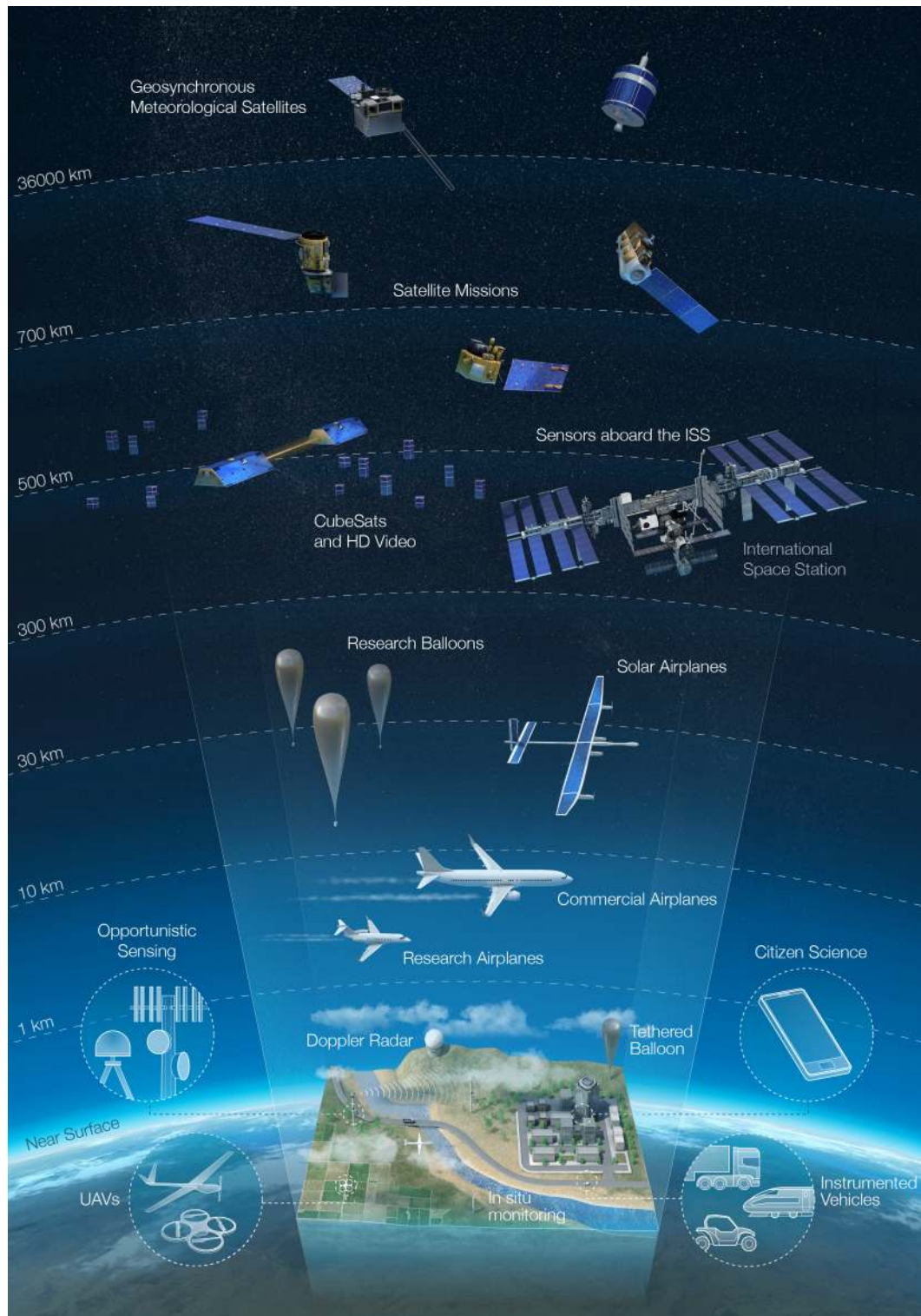
Figure 2. An Earth-observing “system of systems” for revolutionizing our understanding of the hydrological cycle. This multi-scale, multi-resolution observation strategy is not really a concept, as the technology exists and is largely in place now. Supporting traditional space-based satellites, there are now a range of orbital options from commercial CubeSats to demonstration sensors on-board the International Space Station. Beyond orbiting EO systems, technological advances in hardware design and communications are opening the skies to stratospheric balloons and solar planes, as well as an explosion of UAV-type platforms for enhanced sensing. At the ground level, the ubiquity of mobile devices are expanding traditional in situ network capacity, while proximal sensing and signals of opportunity are opening up novel measurement strategies.
