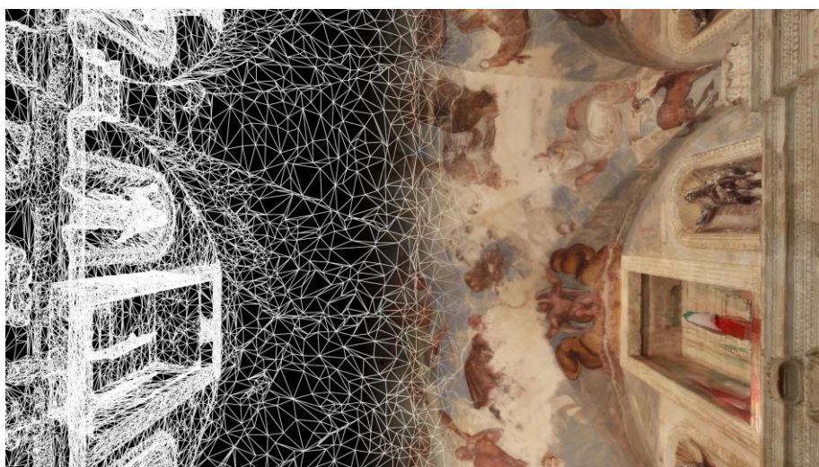
Fig. 18: Rendering of 3D Model Wireframe and Textured, a detail of the vault
