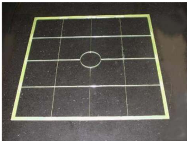
Fig. 28. The thin insulating spacer used to prevent electrostatic deformations of the gaps. The central pattern corresponds to the beam area.
