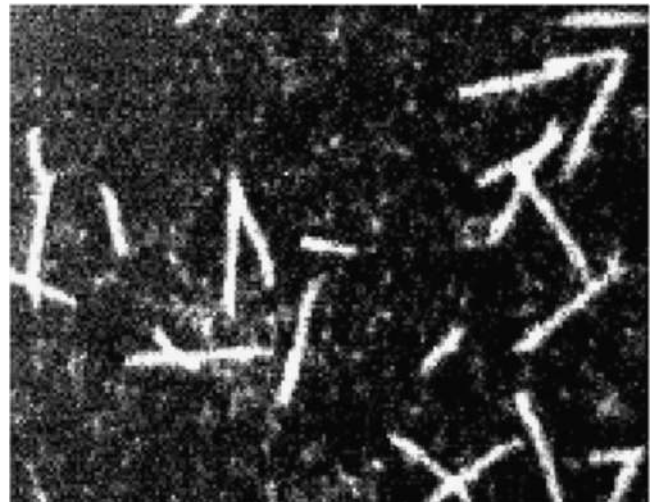
Fig. 74. Neutron conversions in 3 He recorded with a solid state camera from the photon emission in a multi-GEM amplifier.
