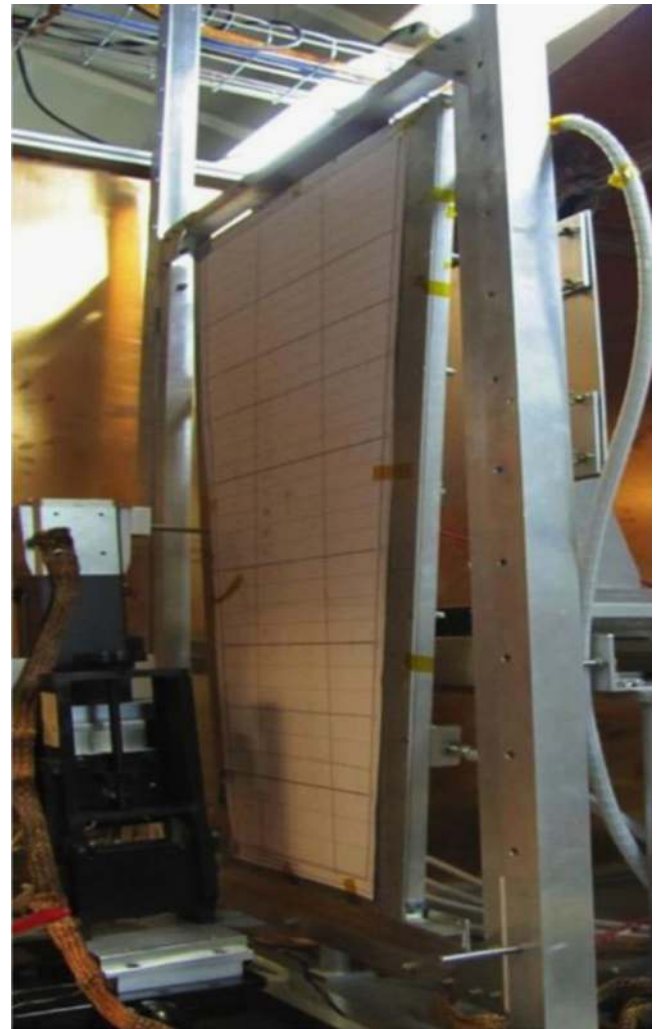
Fig. 34. A large GEM prototype for the CMS forward muon upgrade. The detector is about one meter high.
