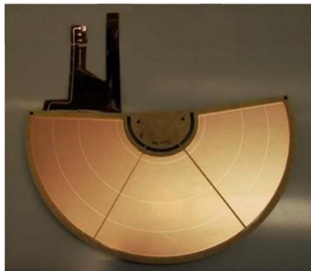
Fig. 30. Half-moon shaped GEM for the TOTEM tracker.
