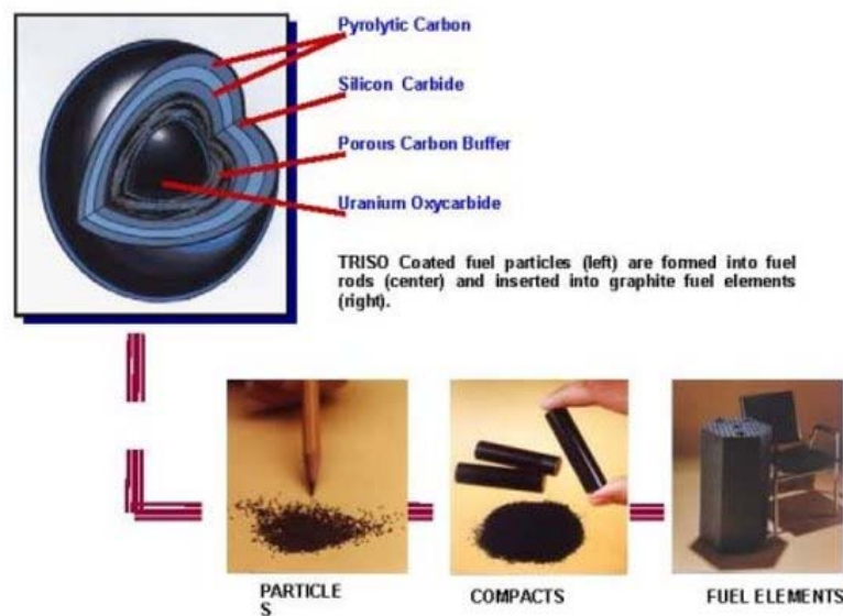
Figure 3: GT-MHR TRISO coated particle fuel
