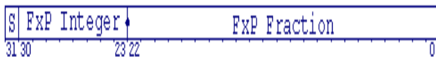
Fig. 1 IEEE standard single precision floating point representation and the 32-bit LNS format
