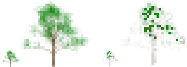
Figure 3 GPC-based 361x extreme antialiasing (left) and conventional hardware supported 16x antialiasing (right). Images are also shown magnified at 400% for illustration purposes.
