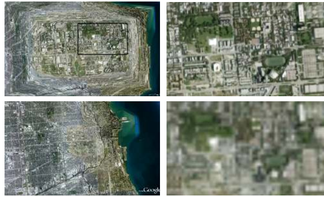
Figure 14. GPC reference image and frame resampled from it (top) and corresponding PPC image and frame for comparison (bottom).
