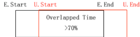
Fig. 4. Audience detection algorithm: if intersection of duration of user stop and duration of the event is greater than 70 percent and user's home is not the same as the event location, then we mark the user as audience of the event
