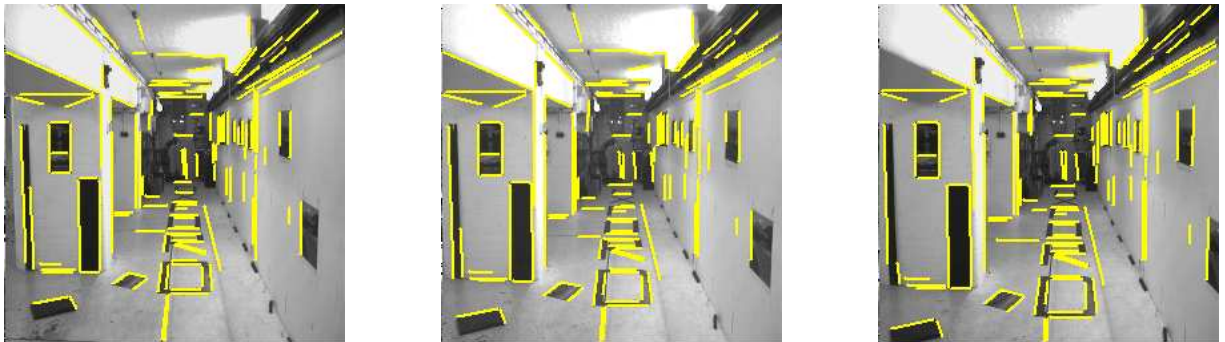
Figure 26: Three view line matching III : The images are 512 \times 512 pixels. There are 282/285/285 line segments in the first/second/third views. Of these 130 are matched, all the line matches are correct.
