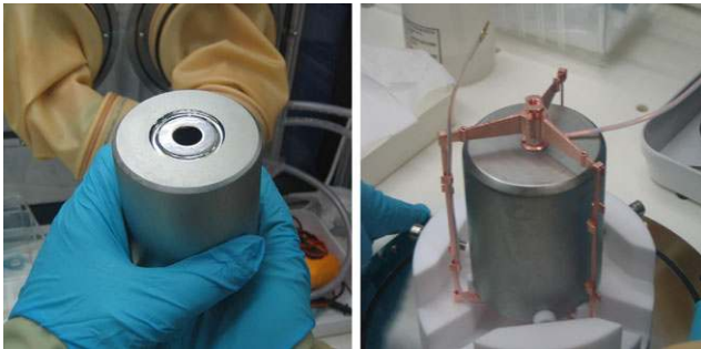
Fig. 5 Left: A Phase I detector after reprocessing at Canberra, Olen. The conductive lithium layer ( n^+ contact) and the boron implanted bore hole ( p^+ contact) are separated by a groove. Right: The detector is mounted upside down in a low-mass holder (groove no longer visible)
