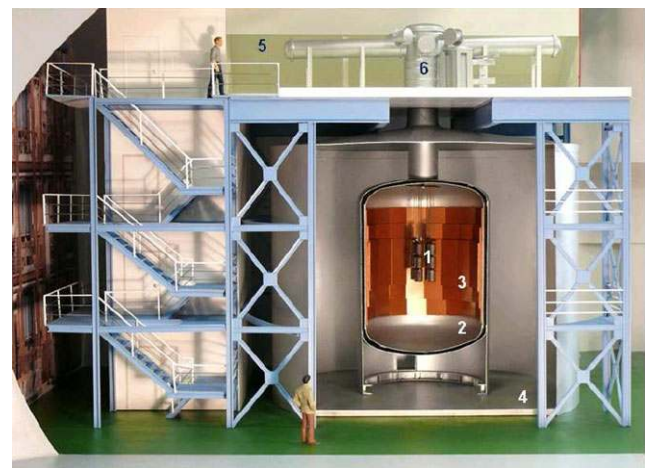
Fig. 1 Artists view (Ge array not to scale) of the GERDA experiment as described in detail in the following sections: the germanium detector array (1), the LAr cryostat (2) with its internal copper shield (3) and the surrounding water tank (4) housing the Cherenkov muon veto, the GERDA building with the superstructure supporting the clean room (5) and the lock (6, design modified). Various laboratories behind the staircase include the water plant and a radon monitor, control rooms, cryogenic infrastructure and the electronics for the muon veto
